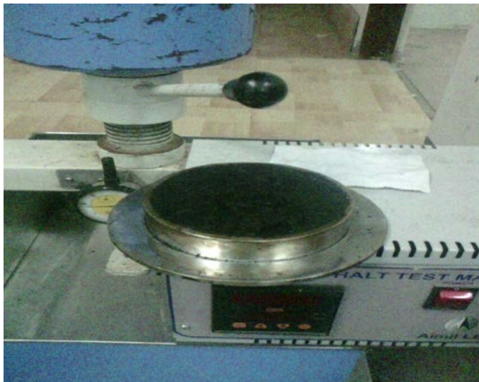
Figure 3. Mastic Asphalt Test Machine with Specimen
